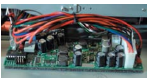
The latest DC to DC power adaptors avoid the use of inverters and mains voltages. Developed for commercial trucks, they are over 95% efficient and have high input ranges 6v to 32v for reliable 12v or 24v operation.
