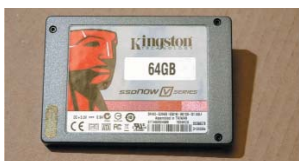
Solid state hard drive - no moving parts to break or skip
