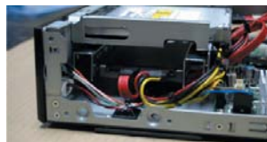
All cables secured with cable ties
